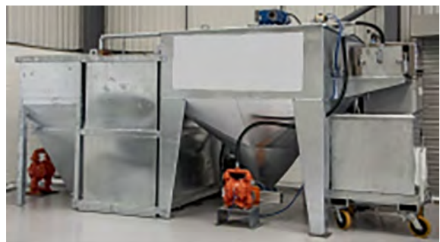
Figure 15 Waste water/slurry management system
